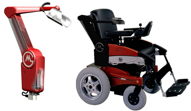
Fig. 5. The arm support Mark III, called Armon [19]. On the left the product in a semi-see-through view, showing the springs inside the base links and the balancing adjustment actuator in the box; on the right the product as fitted to a wheelchair.
