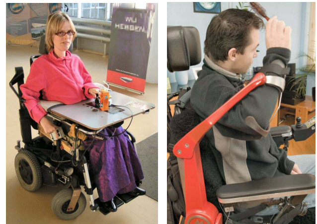
Fig. 6. The Armon in lowest and highest position. This range is sufficient for several important activities of daily living.
