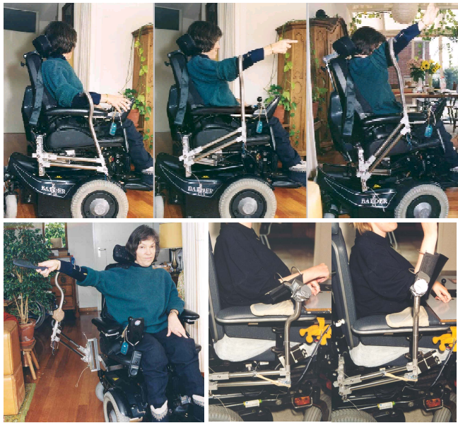
Fig. 2. Prototype of the arm support, Mark I. This prototype was manufactured to validate the principle of full balancing while only partially supporting the arm mass [2]. Top: This subject (SMA II) is capable of raising her arm. Bottom left: Also moving out is possible. Bottom right: This subject (SMA I) has difficulties in raising her arm.
