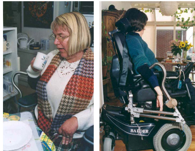
Fig. 3. Prototype of the arm support, Mark I, showing some problems encountered with it: Fitting design: (left) Interference between mobile arm support and fixed arm rest prevents movement from the hand to the face, (right) dead point where control is lost and the arm is locked.
