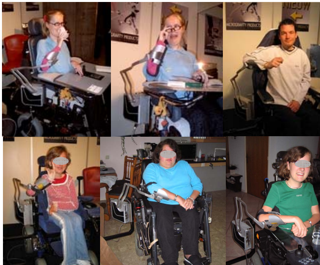
Fig. 4. Prototype of the arm support, Mark II. This prototype was manufactured to evaluate the design in a home or clinical setting by trying it out on a larger number of patients (around 16) so as to gain user feedback [17].
