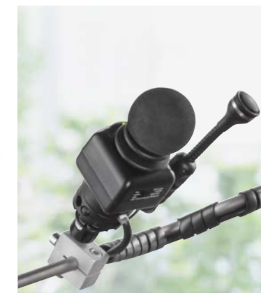
Electrical or manual chin control CODE/Article No.: 565/1074111 (electrically) or 810/1072890 (manually) The chin control is mounted on the push bar of the wheelchair. The operating elements (chin control joystick, on/off button and mode-key), including the holder can be swivelled side to side electrically or manually by hand.
