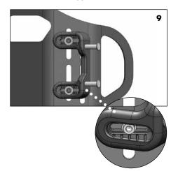
4. Wheelchair frame widths can vary from chair to chair. If you have any trouble aligning the mounting brackets with the attachment pins, you can easily adjust the width of the Java Back to fit perfectly.
