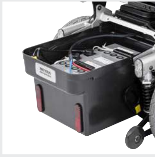
Service-friendly Simple battery maintenance thanks to pull-out battery box
