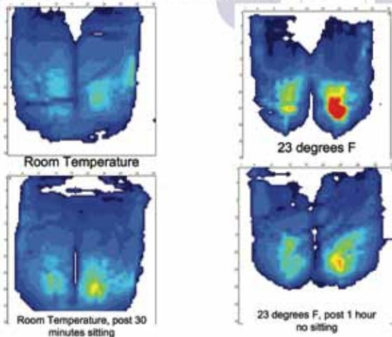
Cushions that utilize temperature sensitive materials for skin protection will have varying performance characteristics relative to cushion temperature. They may not be safe to sit on if allowed to cool excessively, and may bottom out over time when warmed.
