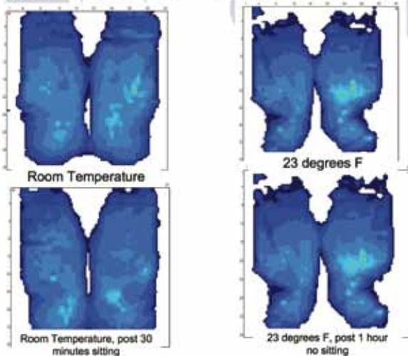
The Ride Forward Cushion shows consistent and safe performance across a broad range of temperatures. Additionally, the spacer fabric cover helps to reduce heat and moisture at the sitter interface.
