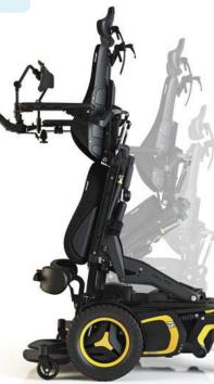
When sitting and driving, these support wheels retract completely, allowing a top speed of 12 kmh.
