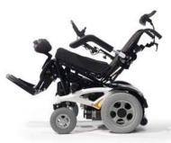
requirements. It also features a completely new integrated seat sliding system to enable the user to get closer to a desk or table.
